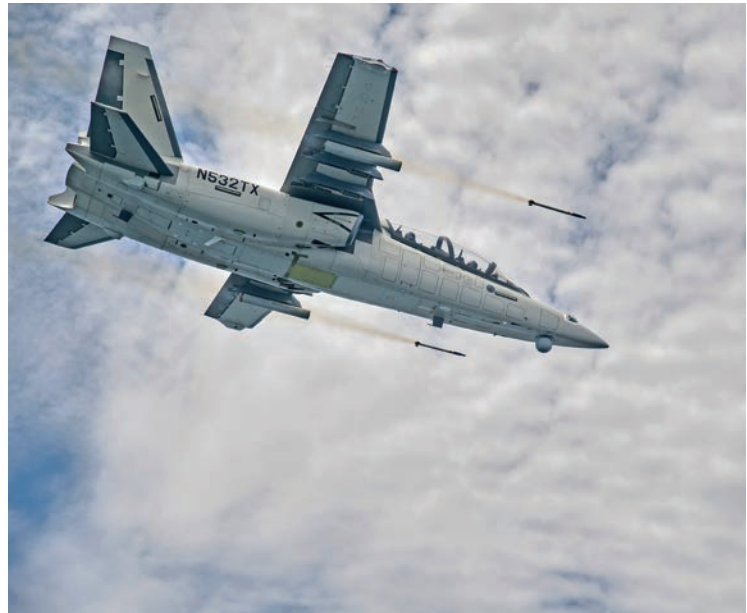
TWO LARGE BELLY BAYS can handle any number of sensors or fuel tanks (top left). The six wing-mounted pylons (above) can carry various sensors, fuel tanks, or weapons, including laser-guided missiles and rockets, GPS-guided bombs, and .50-caliber machine guns spewing 1,100 rounds per minute. Need more range? Hellfire missiles work, too. This Scorpion can sting! The red trigger button on the back of the control stick unleashes the weapons (left). The HOTAS stick, thrust levers, HUD, and yellow-and-black-looped ejection seat handle (opposite, top) give the cockpit a military look. But the big Garmin display and dual touchscreens show the civilian side of Scorpion. The backseater's big display primarily shows sensor data (opposite, bottom).
